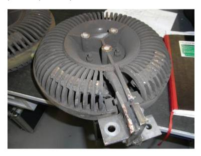
Fig 2 below shows the very limited clearance between the inductor and the pan well roof:
